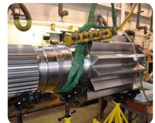
Pinion Gear Journal Bearing Defect Repair
